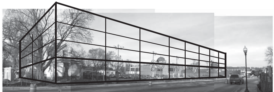
5.3 Completed block perspective is now ready to be used to develop building sketches.
